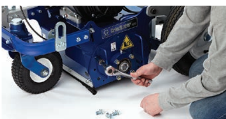
1. Loosen four bolts
