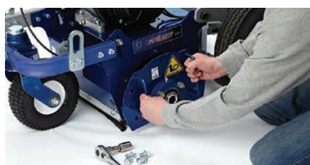
2. Remove bolts and door
